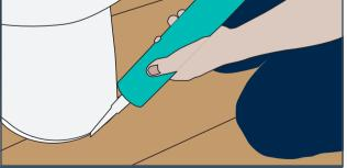
11. For splash areas such as bathrooms, waterproof skirting/scotia/ trims can be used. Cut the flooring around your WC base leaving a 6-10mm expansion joint. 100% Silicone sealant can be used to fill in the gap. Silicone can be used in small areas such as around sink pedestals but should not be used on large areas as it will restrict the expansion and contraction of the flooring causing the joint edges to fail.
