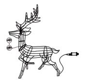
Fasten together the deer head (1) and the deer body (2). Rotate the C buckle on the upper part of the deer outwards, then press the wire under it to tighten.
