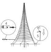
Insert the ground stakes (5) and the ground insertion rod (3) into ground to fix the ends of the 6 ropes and the whole product.
