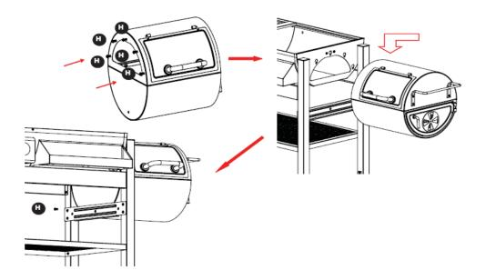
Fix the Temperature gauge 37 on the Gas grill lid 40. Fix the Handle 35 and the heat shield 41 on the Gas grill lid 40 using M6\*15mm bolts 41.
