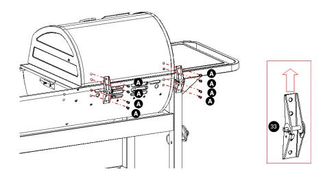
Fix the Hinge  $\ensuremath{\mathfrak{B}}$  on the charcoal grill using M6\*12mm bolts (A) .
