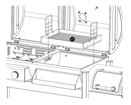
Fix the Warming rack 🚳 in the Gas grill and Characoal grill using M6\*35mm bolts ①.
