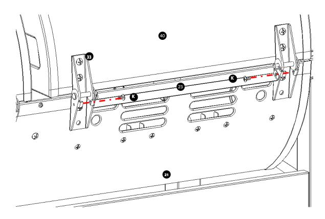
Insert the Grease Cup Wire Hook through the grease drain hole on the bottom of the Cabinet . Place the Grease Cup into the Wire Hook.
