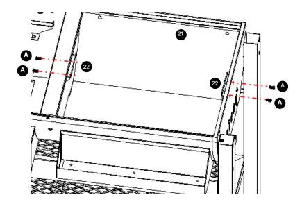
Fix the Side burner control panel <sup>2</sup> on the Side burner assembly <sup>1</sup> using M4\*8 bolts <sup>B</sup>. Fix the Side burner assembly <sup>1</sup> on the Grill cabinet assembly <sup>2</sup> using M6\*12 bolts <sup>A</sup>.
