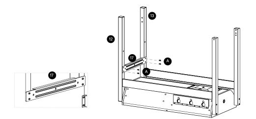
Put the bottom shelf <sup>6</sup> to the Right front leg <sup>12</sup>, Right rear leg <sup>13</sup>, Left front leg <sup>8</sup> and Left rear leg <sup>7</sup> using M6\*12mm bolts <sup>A</sup>.
