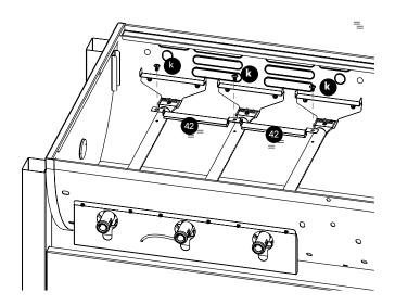
Put the ignition wire on the burner 2 into the igniter on the Control panel assembly 5.
