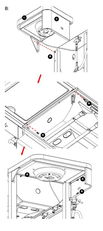
Fix the valve on the side burner control panel  $^{2}$  using M4\*8 bolts  $^{1}$
