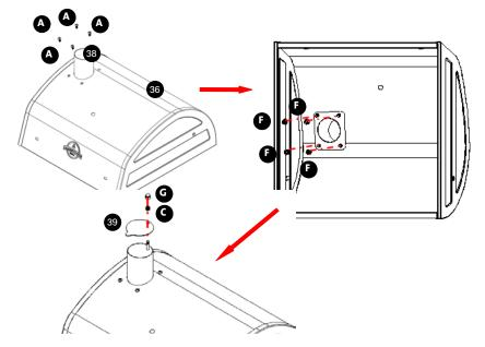
Fix the Temperature gauge ③ on the charcoal grill lid ⑥ . Fix the Handle ⑧ on the charcoal grill lid ⑧ using M6\*15mm bolts Ħ .
