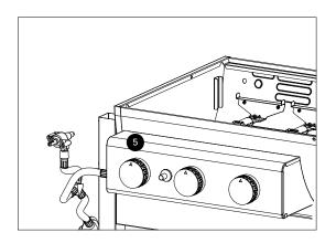
B: Make sure the tip of the valve is completely inside the burner venturi.
