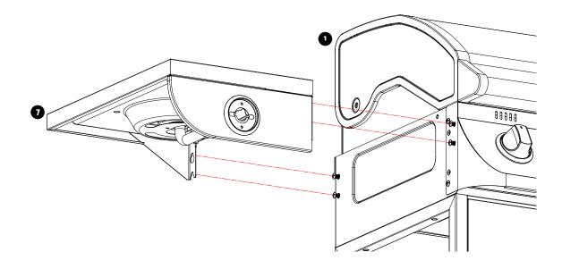
Align the 12mm bolts A properly with the Side table assembly . Hang the Side table assembly to the Grill assembly . Secure the bolts tightly by screwdriver after the alignment is done.
