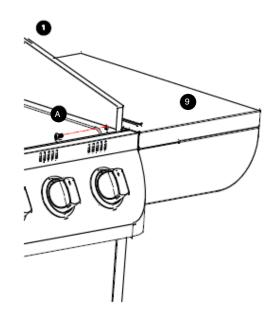
A: Loosen the two pre-assembled screws between the side burner and the Side burner assembly 🕐.
