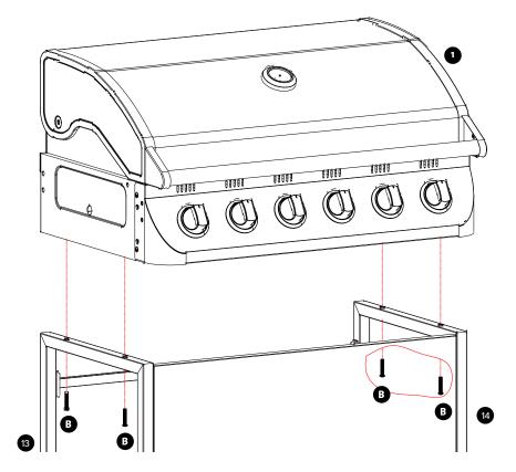
Apply 8 of the 12mm bolts (4) to the left and right side of the Grill assembly (1). Have half of the bolt threads go into the bolt holes. Do not tighten the bolts at this stage.
