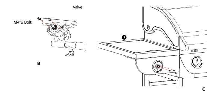
D. Align the side burner venturi against the valve. Make sure the valve tip goes into the burner venturi completely with good alignment. Then tighten those two screws loosened at procedure A on the side burner after the alignment.
