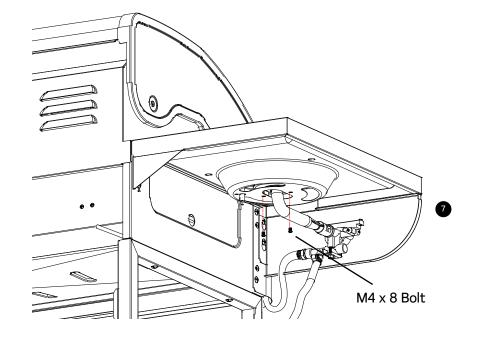
E. Install the Side burner electrode wire to the side burner electrode and igniter. Connect the black end to the electrode of the side burner assembly . Then connect the red end to the igniter of the side burner valve.
