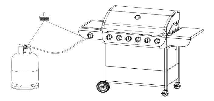
Always place the gas bottle at the side of the appliance. The gas bottle should be sited as far away from the appliance as possible without straining the hose. The hose length should not exceed 1.5m.
