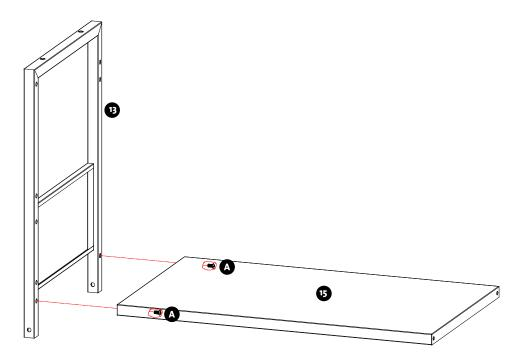
**Step 2**Put the Cart - Right side panel assembly 4 on the Bottom shelf assembly 5 using 12mm bolts 4.
