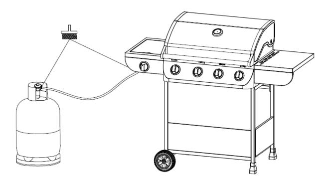
Always place the gas bottle at the side of the appliance. The gas bottle should be sited as far away from the appliance as possible without straining the hose. The hose length should not exceed 1.5m.
