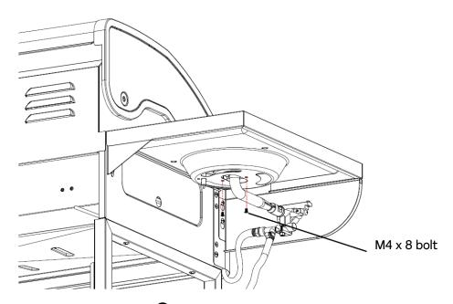
E. Install the Side burner electrode wire to the side burner electrode and igniter. Connect the black end to the electrode of the side burner assembly. Then connect the red end to the igniter of the side burner valve.
