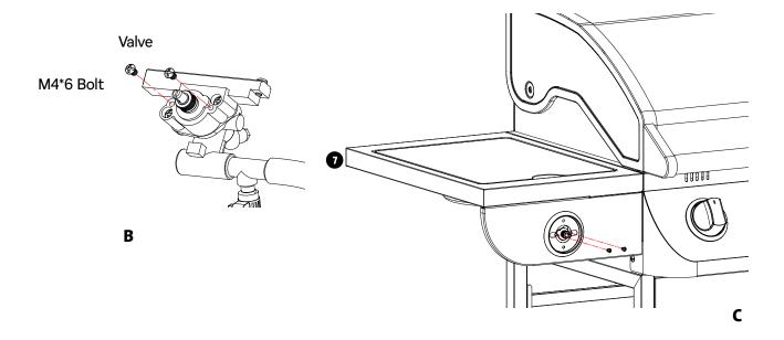
D. Align the side burner venturi against the valve. Make sure the valve tip goes into the burner venturi completely with good alignment. Then tighten the two screws loosened at procedure A on the side burner after the alignment.
