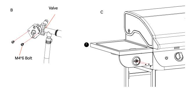
D. Align the side burner venturi against the valve. Make sure the valve tip goes into the burner venturi completely with good alignment. Then tighten those two screws loosened at procedure A on the side burner after the alignment.
