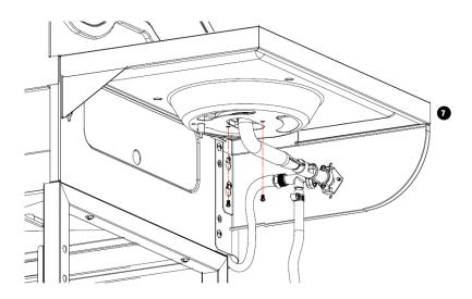
E. Install the side burner electrode wire to the side burner electrode and igniter. Connect the black end to the electrode of the side burner assembly. Then connect the red end to the igniter of the grill assembly.
