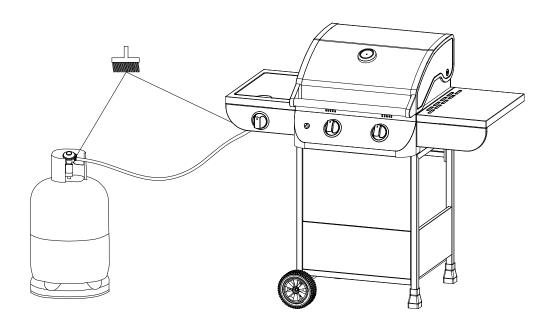
Always place the gas bottle at the side of the appliance. The gas bottle should be sited as far away from the appliance as possible without straining the hose. The hose length should not exceed 1.5m.
