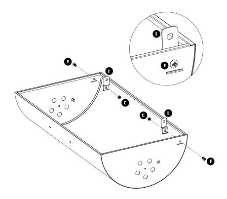
Step 7 Put the washer () between the lid handle () and the lid (). Then fix the lid handle () on the lid () using 10mm bolts ().
