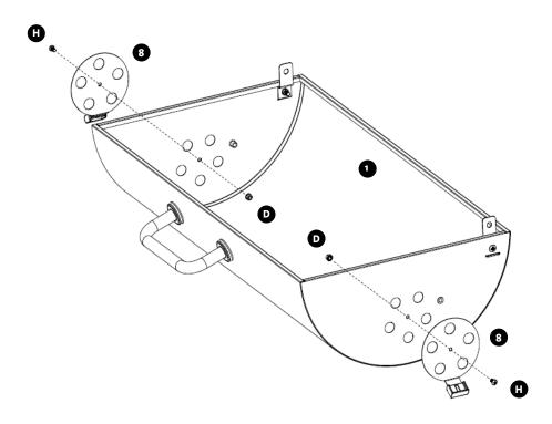
Fix the lid supports **①** with the fire bowl **2** using 15mm shoulder bolts **③**.
