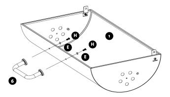
Step 8 Fix the dampers (8) on the lid (1) using 10mm bolts (H) and M5 nuts(D).
