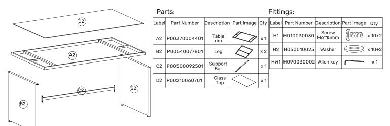
Step 1: Use screws (H1) and washers (H2) to fix the leg (B2) to the table top (A2). Repeat these steps to the other support and fully tighten all the screws.
