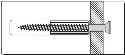
These come in various sizes and are made from plastic or sometimes wood fibre.
