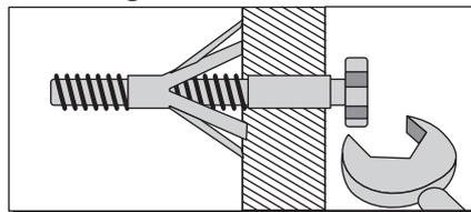
For use when fitting or supporting heavy loads such as shelving, wall cabinets and coat racks.
