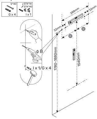
Measure the mounting hole distance of the cabinet, as shown. Mark the installation position on the wall with a pencil and keep it level. Drill holes and insert expansion tubes into the wall.
