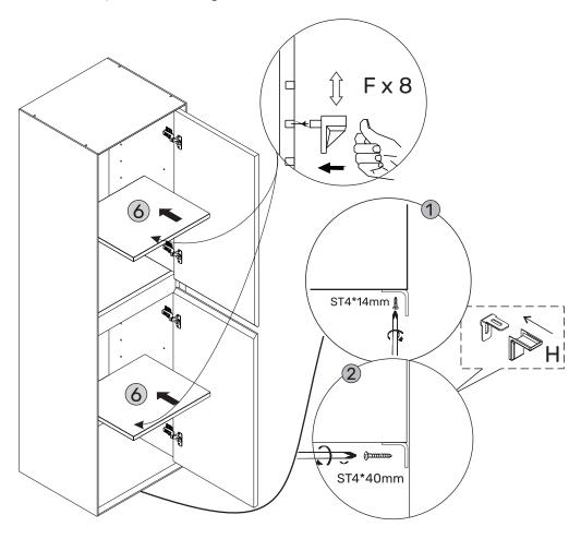
Place panels 6 in the unit and secure using bracket F. Fix the bottom panel onto the wall with the bracket, using ST4\*14 and ST4\*40 screws.
