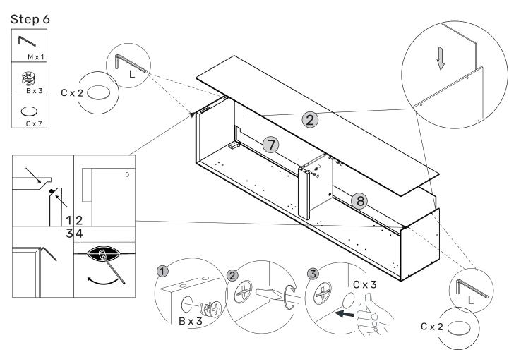
Connect panel 2 to panels 3, 4 and 5 using Allen Key M. Fix together tightly with B and place cover C on top of B.
