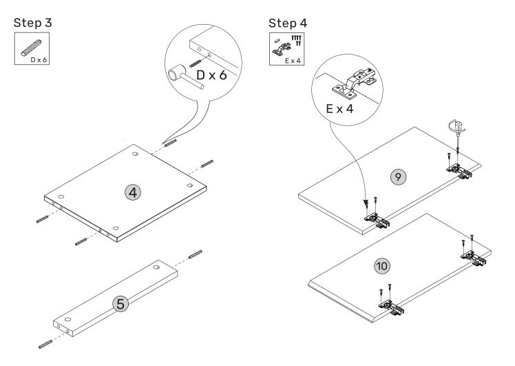
Insert wooden dowels D into panels 4 and 5.
