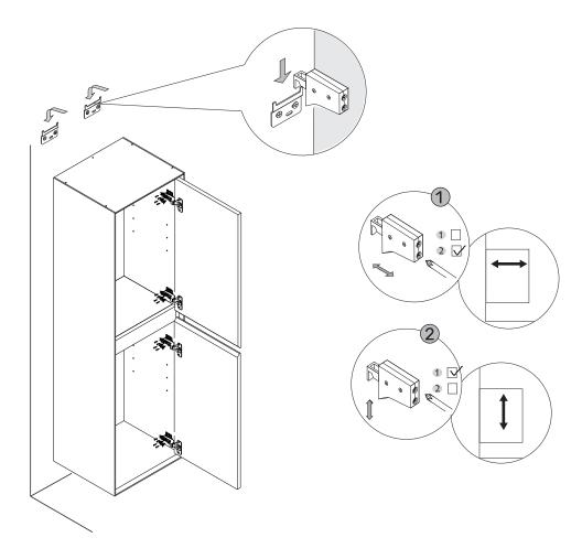
Put the unit on the wall and adjust the lifting code as shown.
