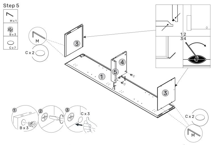
Connect panel 3 to panel 1, using Allen Key M. Attach panels 5 and 4 onto panel 1 and fix in place using B. Then place cover C on top of B.
