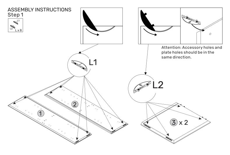
Insert L1 into panel 1 and panel 2. Insert L2 into panel 3.
