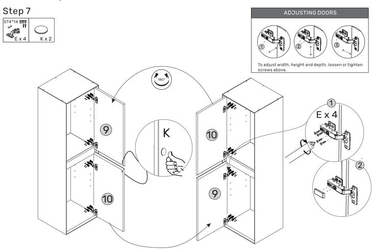
Attach panels 9 and 10 onto side panel 1 or 2 (depending on which way you want the door to open). Adjust the hinges as shown. Affix K on the corner of the door.
