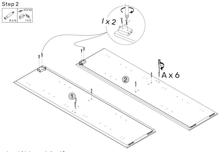
Insert A into panels 1 and 2. Assemble part of hanger I on panels 1 and 2, using ST4\*30 screws.
