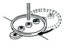
Untighten fixing screw and bracket will adjust to fit the majority of toilet pans.
