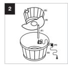
Attach the tube (F) to the nozzle on the pump (H). Then place pump into the lower barrel (G). Be sure to route the power cord of pump through the notch on the lower board.
