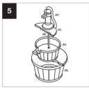
Fit the groove on the upper board (C) onto the edge of the upper barrel (D) to attach the two pieces. Then, connect the tube (B) to the outlet nozzle on the upper barrel.
