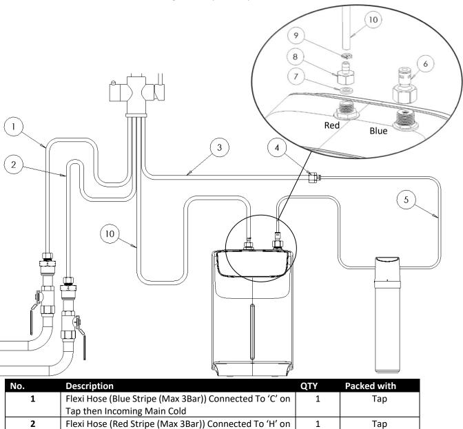
For servicing purposes, the services provided by the customer should have means of isolation. These should terminate with  $\frac{1}{2}$ " BSP male fittings to accept the tap flexible tails (1 and 2).
