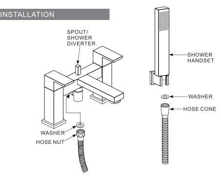
Insert a washer into the cone end of the hose and screw to the handset.
