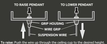
To lower: Press the wire grip into the housing to release the wire. Once at the desired height release the wire grip Coil excess wire inside the ceiling cup.
