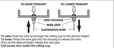
Once at the desired height release the wire grip Coil excess wire inside the ceiling cup.
