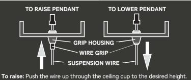
To lower: Press the wire grip into the housing to release the wire. Once at the desired height release the wire grip Coil excess wire inside the ceiling cup.
