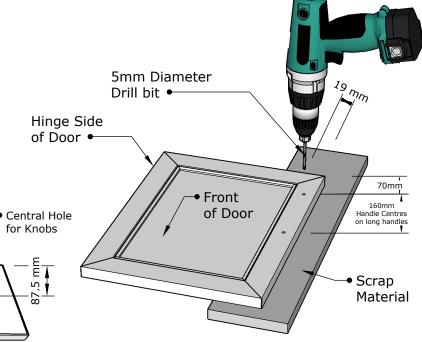
**Guide:** There are no rules for where the handles need to be - it is up to your personal choice. However, as a guide, a hole 70mm from the top of the door (for base units) works well. And fitting handles in the middle of drawer fronts works best.
