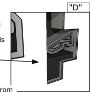
"A" - Turn this screw to adjust the fronts from side to side (This should be rarely needed)
