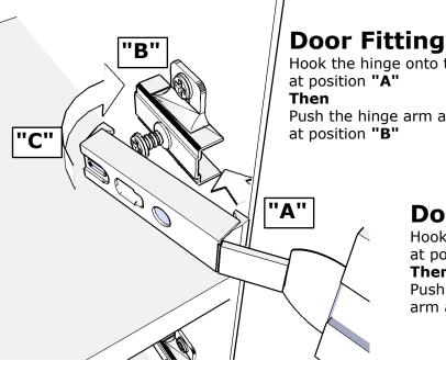
Hook the hinge onto the front of the hinge plate at position "A"
