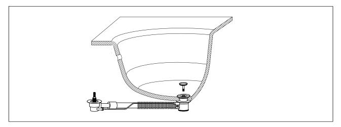
Adjust length of flexi pipe to suit installation. Insert the control valve from the underneath of the bathtub. Insert the nut from the dome and rubber washer to the surface of bathtub and eventually over the valve lever; Fasten the bolt to fix to the body. Tighten the bolt with a wrench if required. (DO NOT APPLY EXCESSIVE FORCE)..
