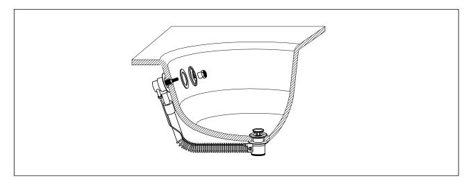
Cover the handle onto the valve lever. Fasten the screw.
