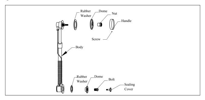
Put the body on the bottom of the bathtub. Insert the bolt from the rubber washer of thedome to the bathtub surface. Fasten the bolt manually to fix the body. Tighten the bolt with a wrench (DO NOT APPLY EXCESSIVE FORCE).
