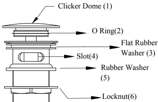
1. Unscrew the locknut (6) and remove the rubber washer (5).
