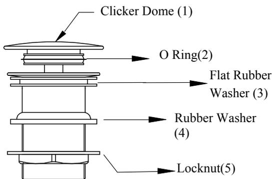
1. Unscrew the locknut (5) and remove the rubber washer (4).
