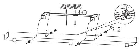
Using the connector block supplied, connect the wires as shown on the diagram below. Step 2 Check that you have correctly identified the house wires, that all connections are tight and that no loose strands have been left out of the connection blocks.
