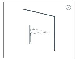
Connect the mirror wires with your main wires, and hang the mounting hole to the screw on the wall.
