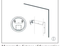
Measure the distance of the mounting hole, Drill holes with a suitable sized drill.
