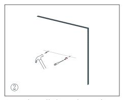
Insert the wall plug and mounting screw into the wall.
