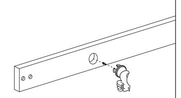
Using the 9mm plastic blanking plugs provided, plug the holes that will not be used to mount the track to the wall.
