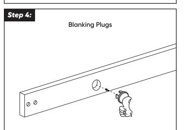
Using the 9mm plastic blanking plugs provided, plug the holes that will not be used to mount the track to the wall.
