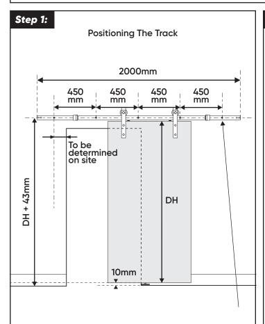
Locate the position of your track. Ensuring the track is level, mark the holes on the wall with a pencil. This will give you a horizontal guide.
