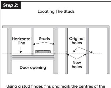
Using a stud finder, fins and mark the centres of the studs along that horizontal line.
