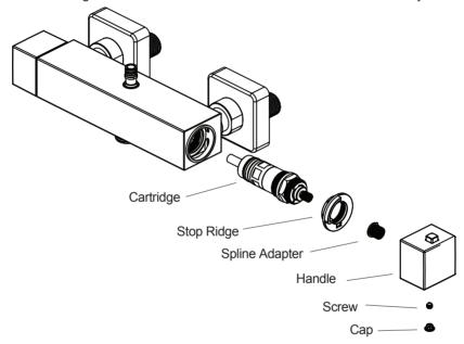
When finishing the cartridge clearance, assemble the Cartridge, Cover, Stop Ridge, Handle, Screw and Cap back into the Valve Body.
