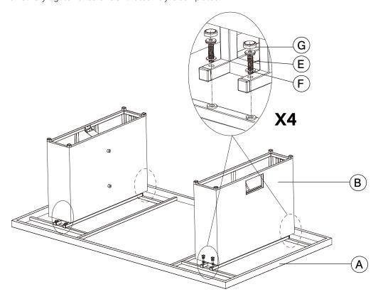
Step 2 Use screws  ${\bf E}$ , washers  ${\bf F}$  and screw caps  ${\bf G}$  to fix the support bar  ${\bf C}$  to the unit. Do not fully tighten all screws until assembly is completed.
