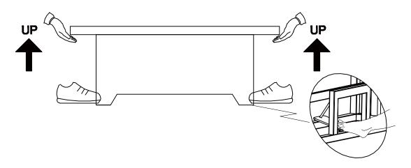
Just step on the rim at the bottom of the table (do not touch the pedal).
