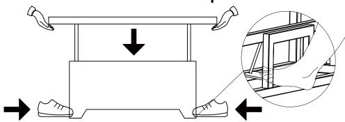
Move the feet onto the pedal and press down. Slowly let down the table top.
