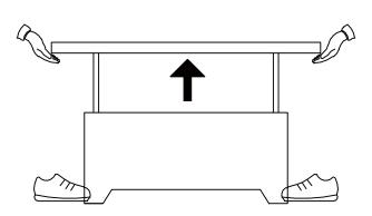
Just step on the rim at the bottom of the table (do not touch the pedal) and lift the table top slightly.
