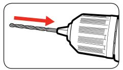
3 Tighten the chuck by turning clockwise.
