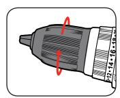
2 Insert the drill bit, making sure it is centred in the chuck.
