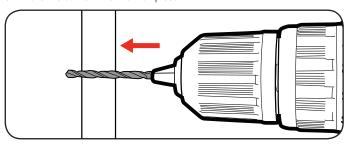
**Note:** Do not force the drill or apply side pressure to elongate the hole. Let the drill do all the work.
