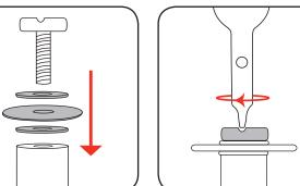
Note: Do not over-tighten the screw as it could result in damage to the cutting disc.
