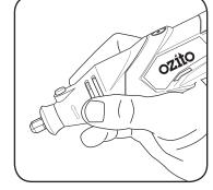
4 For heavy work like cutting or grinding, hold the rotary tool in the palm of your
