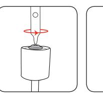
Tighten the screw until the sanding drum sleeve is secured.
