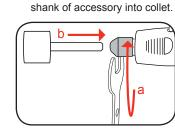
8 Tighten collet nut and check all fittings to ensure they are securely
