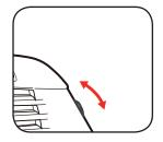
**Note:** The higher the number on the variable speed dial the faster the oscillation frequency of the multi function tool.
