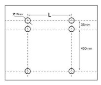
Distance L and M between the fixation points.
