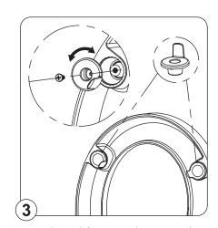
Insert the stabilisers into the seat and test the position. The stabilisers are designed to minimise lateral movement of the seat and provide stability. Change the angle of the stabilisers to achieve a snug fit against the inside of the toilet pan (see figure 3a). Install the screws.
