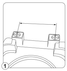
Measure the distance between the pan holes as well as the distance from the pan holes to the front of the pan to determine which sockets on the seat to use. Screw the threaded rods into the required sockets.
