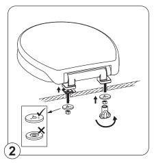
Position the seat onto the pan with the gaskets fitted between the seat and pan. Install the washers and nuts and tighten with the included key. Ensure the washers are facing the correct direction, as shown.
