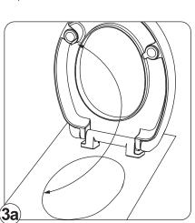
Ensure the stabiliser tabs are as close as possible to the inner rim.
