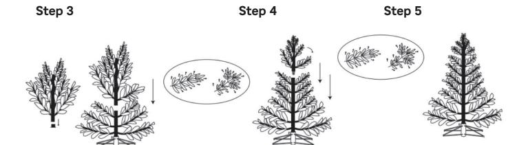
Insert the middle tree section (3) into the bottom tree section and push it down into position. The branches are hinged and will fold down easily.
