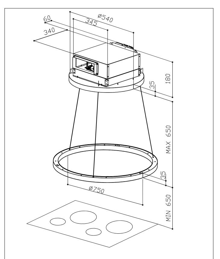
For the installation, create a false ceiling with a niche of diameter equal to 510mm whose minimum height to be reached is 200mm
