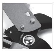
3 Insert the blade hole into the screw, as shown in the image.
