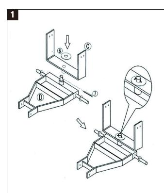
Assemble parts (C) and (D) together, using washers 6 and pins 7 to secure, as shown in the diagrams.
