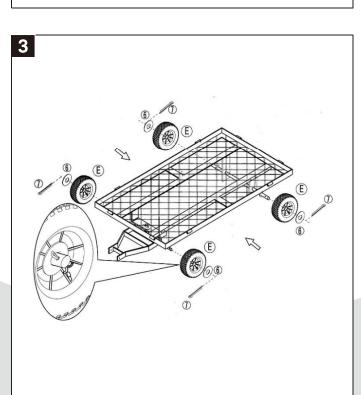
Connect the wheels to the axle bar at the front and back as shown, using washers ⑥ and pins ⑦ to secure each wheel.
