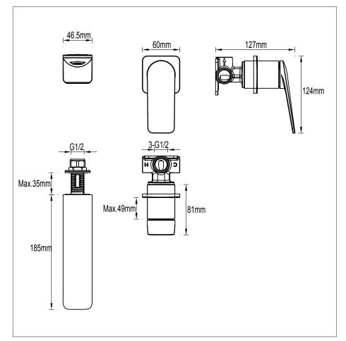
DIMENSIONS: ±5mm Width: 185mm Depth: 60mm Height:124mm
