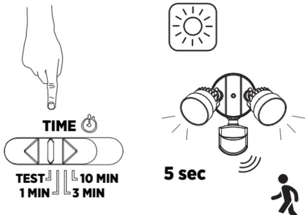
To adjust the detection zone in daylight. When the sensor detects movement the light turns on for 5 sec.
