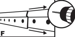
Slide second Hang Track to the right wall of the closet, and then back it away from the right wall until the holes in the two Tracks line up. Repeat Step C to secure
