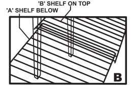
Shelves are fully adjustable and require no cutting. To adjust width, overlap the shelves making sure the shelf labelled A is placed first on the Brackets and the shelf labelled B is placed ON TOP of A.
