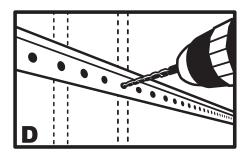
Starting at left side, fasten the FIRST TWO screws into studs (or anchors). Do not fasten behind the first from above. remaining screws until after next step. NOTE: Screws need to be fastened through Track into EACH wall stud.
