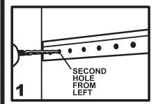
Mark and drill a hole (for a wall anchor) in the second Hang Track hole from the left.
