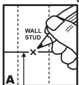
Locate all wall studs on closet wall and mark with an 'X' at the maximum height you require your system to be positioned. **NOTE:** Please consider the maximum height of the Wallstrips to ensure there is ample clearance from the floor.
