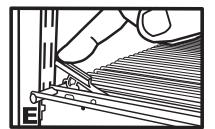
After all shelves are positioned properly, lock shelves into Wire Shelf Brackets by pressing down on the plastic locking clip.
