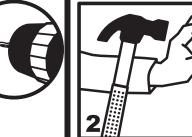
Hammer the wall anchor flush to the wall in the drilled hole.
