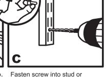
wall anchor. **NOTE:** No screws are needed in top holes of Wallstrips.
