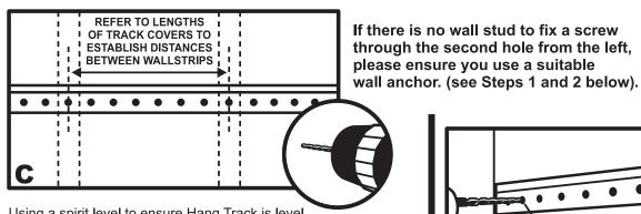
Using a spirit level to ensure Hang Track is level, mark the holes where the wall studs are, then drill a pilot hole. NOTE: If wall studs are not available, please use Plasterboard Plugs (supplied) or suitable Masonry Plugs (not supplied).
