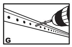
Install screws into studs (or anchors) along Hang Tracks
