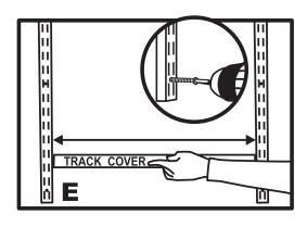
Hang another Wallstrip on the Track anduse one of the Track Covers to space apart (ie 558mm). Drill a pilot hole and fasten screws in bottom hole of Wallstrip. (Use wall anchor if there is no stud). Place Track Cover over Track between Wallstrips. Repeat Step F for one or two more Wallstrips (if space allows).
