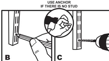
Mark bottom hole of Wallstrip. Fasten screw into stud or Drill a pilot hole into the stud (or wall anchor if no stud is available).
