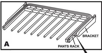
Slide one of the Brackets into the side of the Frame by sliding into the lug as shown in Diag A. Repeat for other side.
