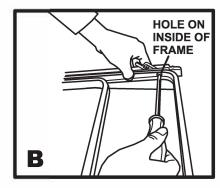
Using a Phillips Head screwdriver, fix the rear of the Frame to the Brackets by inserting and securing the self tapping screws. Insert them through the holes on the inside of the Frame and into the Brackets as shown in Diag B.
